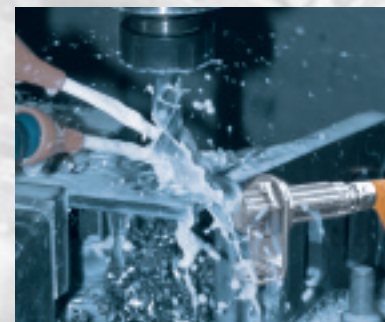
ifm zero-leak sensors are rated IP68 against liquid ingress and can resist the synthetic oils and coolants used in metalworking.
